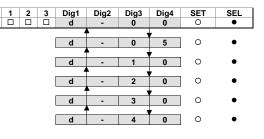
At each pressure of the SEL pushbutton, the different delay levels in ms are visualised in a cyclical manner at the output deactivation and moreover, the relative delay value will be stored When the "d-00" message is visualised the operating mode will be "run", and "rund" in all other cases.
